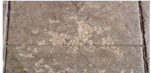
Fig. 3: ASTM C672-98 Scaling Resistance of Concrete Surfaces Exposed to Deicing Chemicals.
